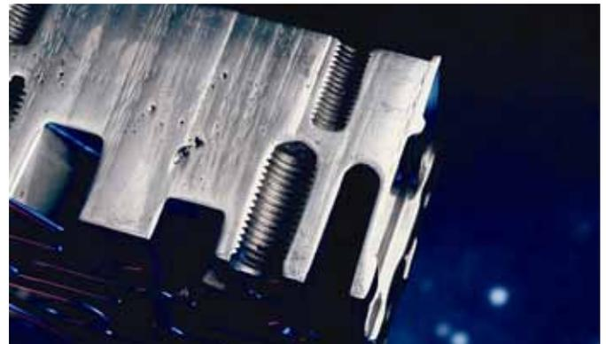
Unfortunately porosities are formed during the die casting process and whilst steps can be taken to reduce the risks, it is extremely difficult to eliminate them altogether.
