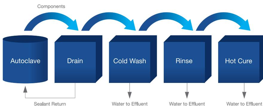
While conventional sealing technologies have made some advances in terms of quality and consistency, over 95% of the total volume of sealant consumed is wasted and goes as effluent in the wash tank during the cold wash process. Only a fraction of the sealant is actually required to seal the porosity. This brings a greater financial burden to companies who are facing ever increasing environmental legislation and costs associated with waste water.
