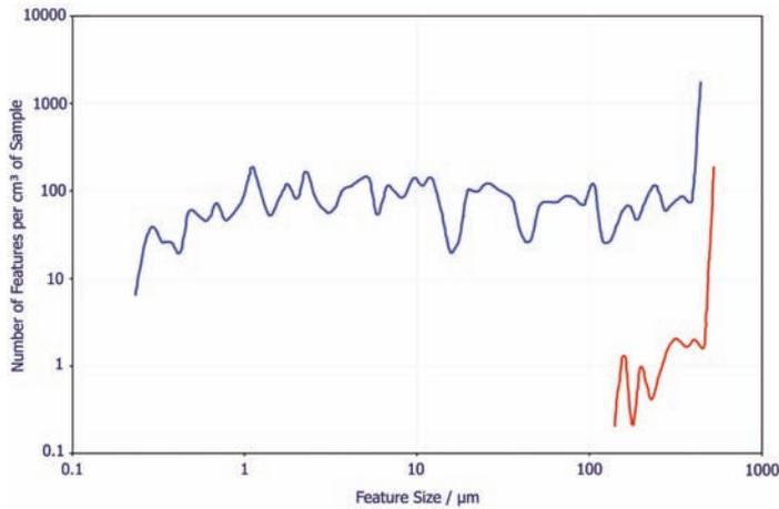
The blue line on the diagram indicates the size and density of the voids (porosity) in a test ring before impregnation.
